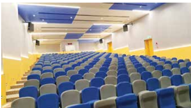
Educational auditorium at Reva Institute of Technology & Management [RITM] Bengaluru Acoustical panelling with a combination of Strand Slim and Slats Surco backed by SynthPF Dissimilar materials create impedance mismatch that results in broadband sound absorption
